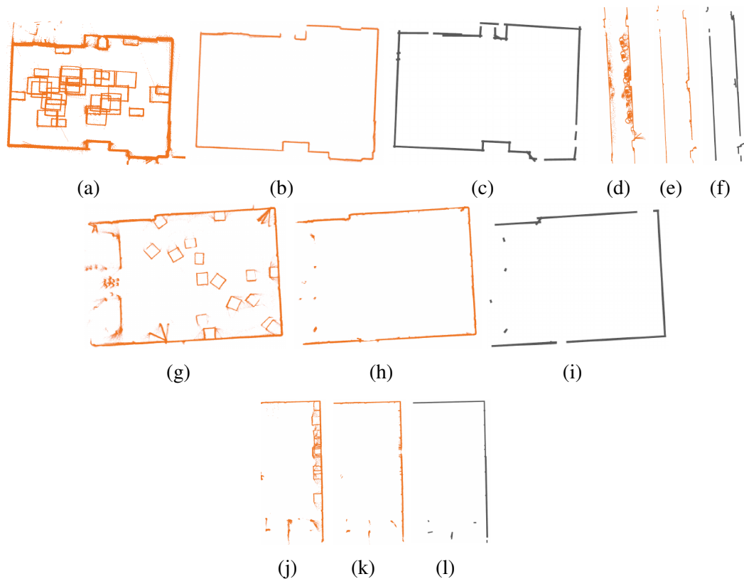
Figure 3.6: Raw data, filtered data, and resultant maps for MIT (a-c), AMRL (d-f), Wall-occlusion (g-i) and Hallway-occlusion (j-l) datasets. Data shown in the left and center columns are aggregates of all deployments and are not stored while the algorithm is operating. The last column is the resultant LTVM which is stored in full, requiring only a few KB. Note the absence of STFs from the final maps, as well as the presence of doorways. In the MIT dataset, some doors were open only once over all deployments. Hallway-occlusion demonstrates the algorithm’s robustness to STFs, as it is able to distinguish the column in the hallway even as it is partially or completely occluded on every deployment.
